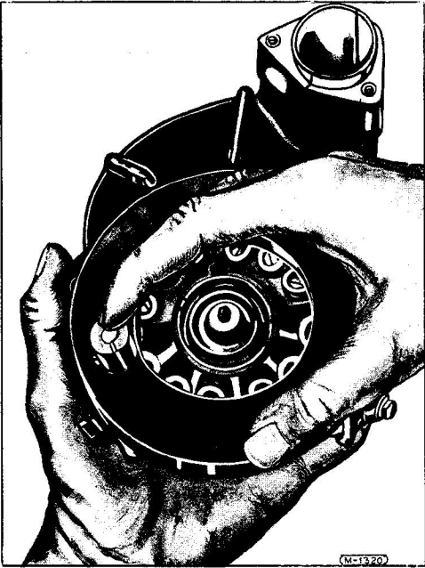
Fig. 2-1 Checking Height of Distributor Block Electrodes
